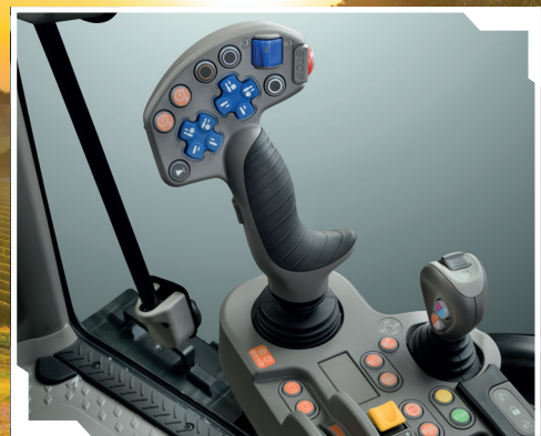
Fully integrated into the seat, the MaxCom armrest is the centre of control of the Fruitteto CVT S and V tractors
