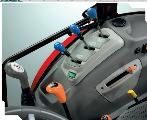
Ergonomic right console with new Easy Lift control.
