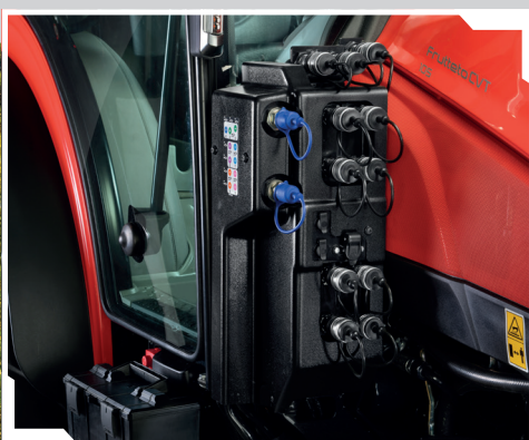
Up to 4 high-flow mid mounted spool valves and up to 3 hydraulic ways duplicated from rear and 2 free returns.
