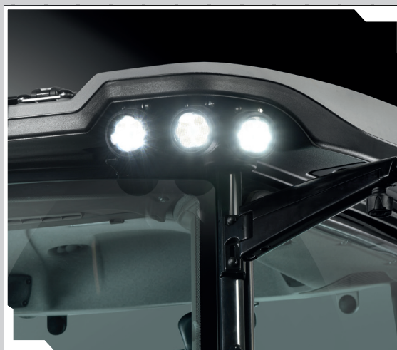
New roof design with up to 12 LED working lights.
