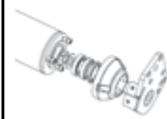
PROFESSIONAL REAR ROLLER Ø 195 mm with 4 taper roller bearings, mud scraper and central body interchangeable with 2 positions: 1) self-cleaning 2) rear (Optional)
