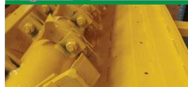
Self-cleaning roller position unloading of mulched product behind the roller for faster working speed
